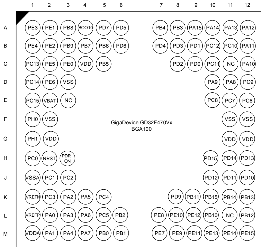
Figure 2-4. GD32F470Vx BGA100 pinouts
