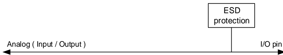
Figure 8-4. Basic structure of Analog configuration
