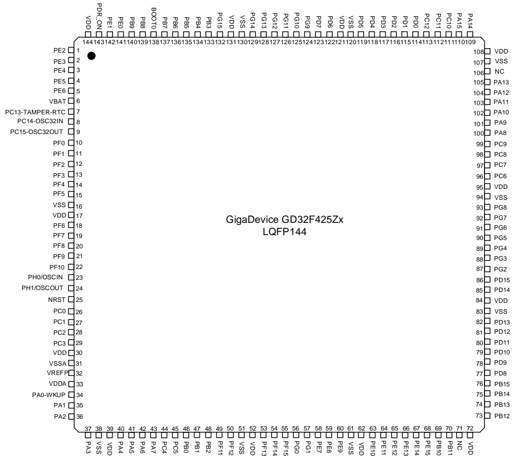
Figure 2-3. GD32F425Zx LQFP144 pinouts
